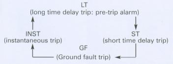
This switch is used to select a measurement mode. Pressing this pushbutton switch toggles in the above order and each measurement mode is indicated both on the LCD screen and corresponding LEDs on the OCR checker. (fig. 1).
