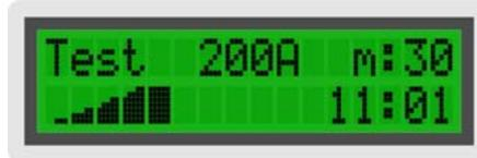
Once the current ramp reaches its maximum value, RMO200 measures the current through the test object and the voltage at the test object for 1s, calculates the resistance from these values, and saves the data at the present memory position.
