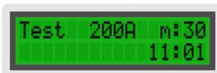
The **Test** menu displays the test current and memory position defined. If one of these values has to be changed, press **STOP** to return to the **Sing** menu.
