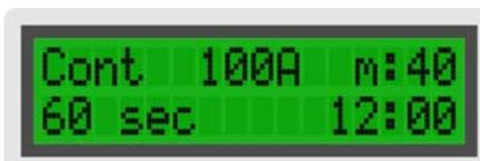
In the **Cont** menu, define a test current, memory location and test current duration time.
