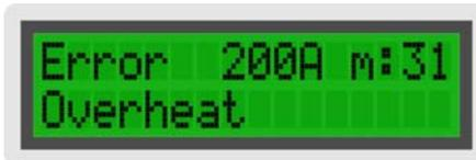
In this case, wait for the test set to cool down and repeat the test.
