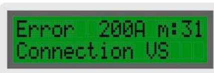
**Note:** Voltage sense cables disconnection, occurred during the test, will cause an erroneous result. The display will not show this as an error message.
