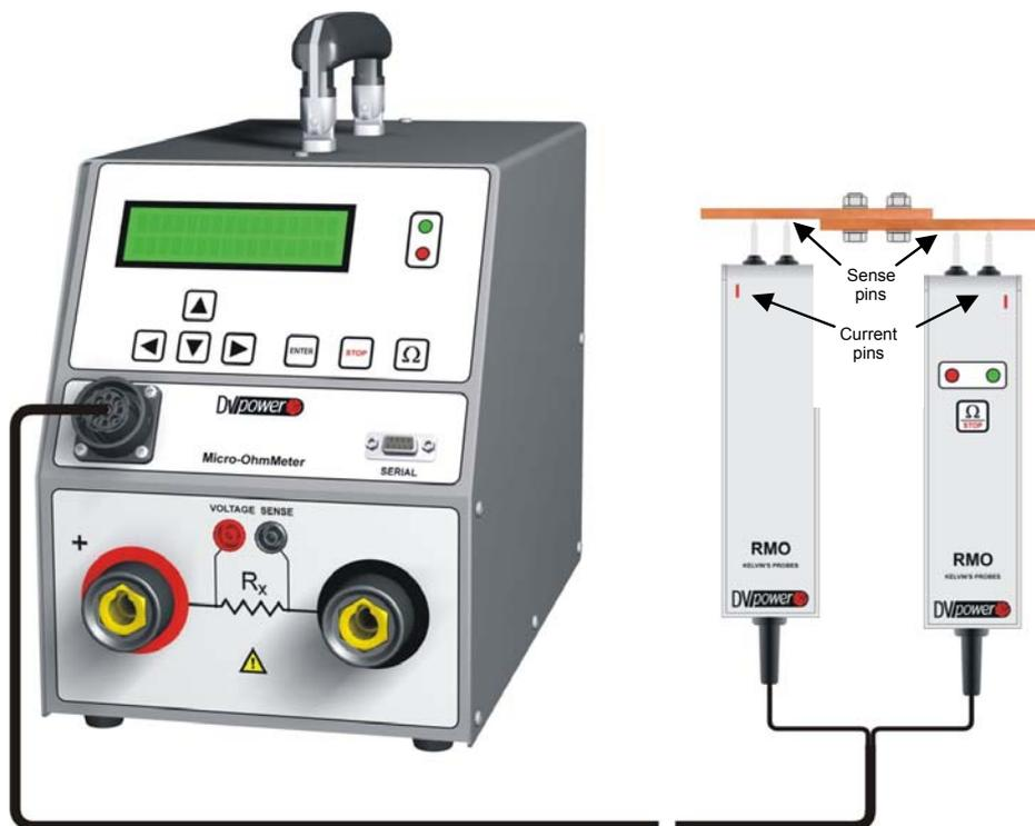
Turn off RMO and plug in the Kelvin Probes to connector on the RMO's front panel.
