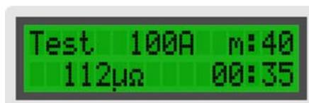
Upon completed test (due to expire of selected time or due to push to the **STOP** button) at selected memory location the last measured result will remain registered.
