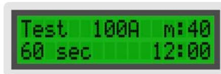
The **Test** menu displays selected test current (here 100A), its duration (here 60 sec) and memory location of the result (here m:40). If one of these values has to be changed, press **STOP** button to return to the **Sing** menu.
