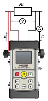
For the contact resistance measurement of a medium voltage circuit breaker with the RMO-H it is convenient to use the cables with the same length. The cables with Kelvin probes (with trigger button) are specially designed for this application.
