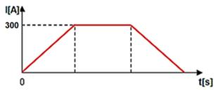
During a test the RMO-H ramps with increasing current before measuring and decreasing current after the measurement. This significantly decreases magnetic transients.
