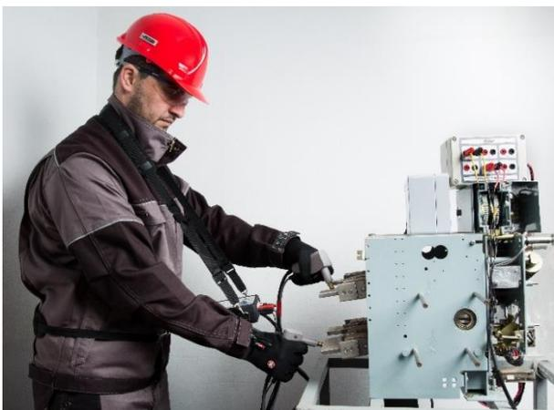
When testing live tank HV circuit breakers with RMO-H a different cables length may be used. The short cable (red cable, 1,3 m) connects the RMO-H to the CB's bushing close to the test person and the device. The long cable (black cable, 3 or 5 m) is connected to a further away positioned bushing on the other side of the breaking point.
