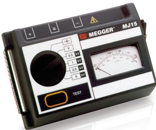
The BM15 and MJ15 are compact 5-kV insulation testers. They are very simple to use and provide a quick and accurate reading of insulation resistance. The instruments use an analog display with a maximum reading of 20 G $\Omega$ . The BM15 is powered by batteries. The MJ15 has an additional hand-cranked generator.
