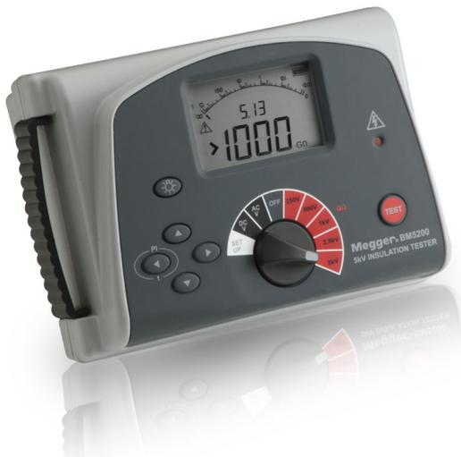
DC insulation tests are performed at 250 V, 500 V, 1000 V, 2500 V, 5000 V. Insulation resistance measuring range is 100 k  $\Omega$  to 1000 G  $\Omega$ . Automatic discharge for capacitive circuits under test is provided and decaying voltage displayed.
