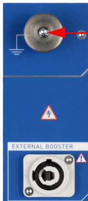
Connect the *CIBANO 500* grounding terminal to the grounding system on site.
