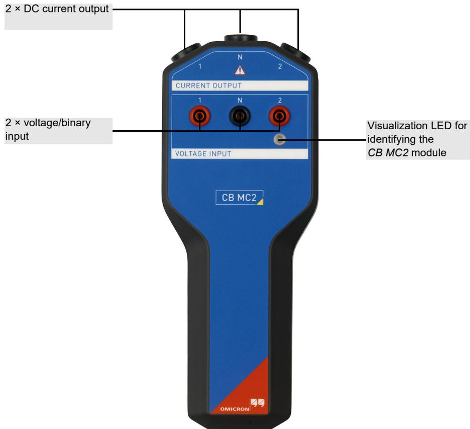
Figure 22-1: Front view of the *CB MC2* module
