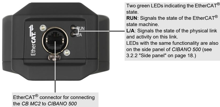
Figure 22-2: Bottom view of the *CB MC2* module
