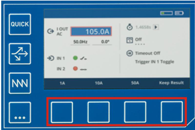
Their functions vary, depending on the screen and the position of the focus. A key's present function is indicated at the bottom of the screen right above the menu key. In some cases these keys act as acceleration keys to set a specific value, in other cases they provide a certain functionality:
