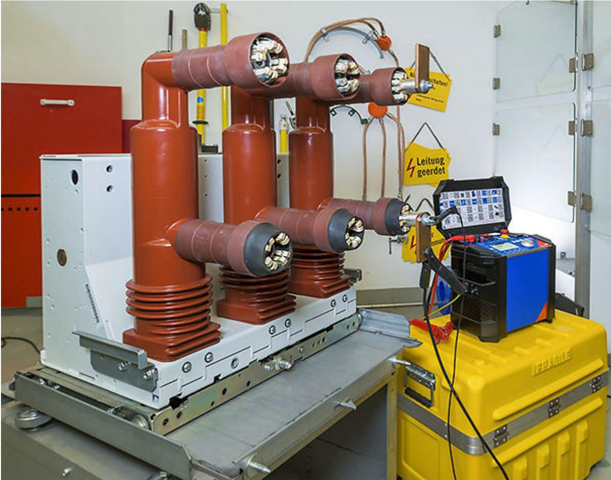
In order to avoid any influence by the contact resistance of the clamps that are connected to the breaker's contacts, it is important to use the four wires (and four contact points!) technique. The current is injected using two wires, the voltage is measured using a second pair of wires.
