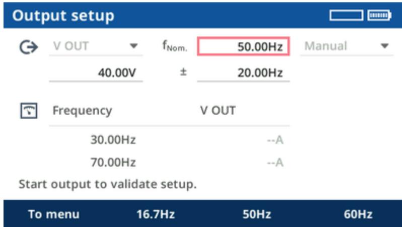
You can test the output configuration by pressing the **Start/Stop** key.
