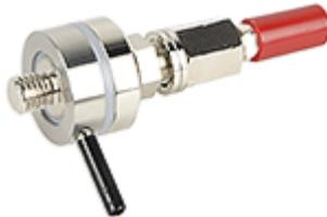
Kelvin clamps also provide the possibility of establishing two independent connections using one clamp, only. The two brackets of the clamp are insulated against each other. Such clamps are ideal when connecting to massive conductors like busbars or connector plates (spades) of a breaker.
