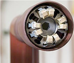
Therefore, in order to measure the total resistance of the breaker, insert stubs substituting the connection points of the busbar (see photo at the right).
