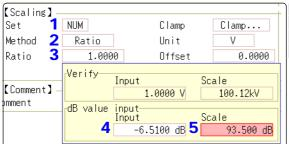
0 dB reference differs depends on the physical quantity. As an example for sound pressure, 20  $\upmu\text{Pa}$  is 0 dB. In dB scaling, the dB value can be directly read; however, it may not be possible to directly read instantaneous values.
