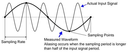
With the Memory function, the sampling rate can be significantly affected by the timebase setting, so care is necessary to avoid aliasing when selecting the timebase. Because the timebase determines the maximum display frequency, the fastest possible timebase setting should be used.
