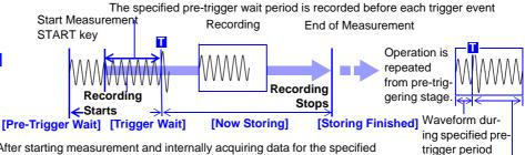
Trigger mode: [Repeat] Pre-triggering enabled
