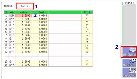
3. In the displayed entry field and physical quantity field, enter 40 dB and 60 dB, respectively.
