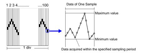
When input waveform variation is slight, the difference between maximum and minimum values (breadth, or width) can be inordinately large if the sampling period is short and if severe fluctuations are present due to noise. This phenomena may be prevented by setting a longer sampling period.
