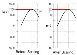
By using the Scaling function, signals from the sensor are acquired as physical values
