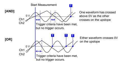
If both [Start] and [Stop] trigger timing criteria are combined, the simultaneous trigger sources are logically ANDed.
