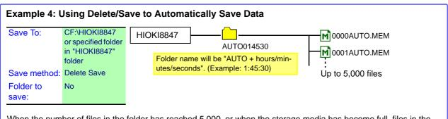
When the number of files in the folder has reached 5,000, or when the storage media has become full, files in the AUTO014530 folder (or specified folder) will automatically be deleted in sequence, starting from the oldest file, and replaced by new files. (Only waveform files are deleted.)
