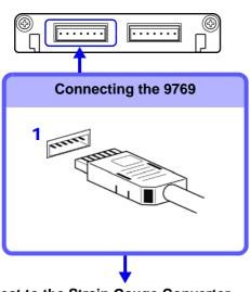
Required item: 9769 Conversion Cable, Strain Gauge Converter
