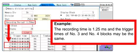
• If triggers occur continuously within an interval shorter than 500  $\mu$ s, the displayed trigger time may indicate a time slower than reality.
