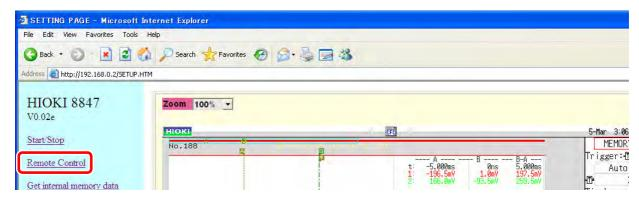
The remote control screen is divided into the instrument display section and operation panel.
