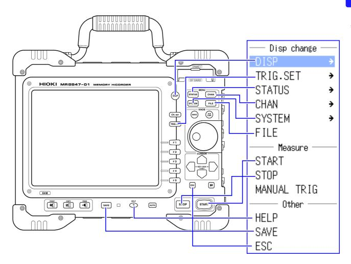
To operate and carry out settings for CH.SET, WAVE, and AB CSR click the icon in the display shown when the mouse is connected. The relationships between the operation keys and icons when the mouse is connected are as follows.
