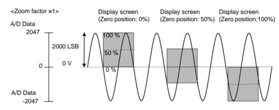
Full-scale resolution for input units at various vertical axis zoom factors (LSB)
