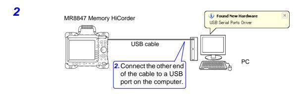
The first time you connect the instrument and computer, perform the following procedure to enable the computer to recognize the instrument.
