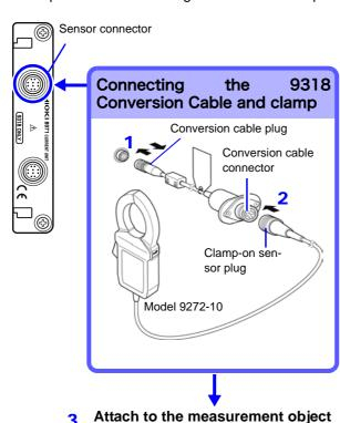
9318 Conversion Cable, 9272 Clamp-On Sensor
