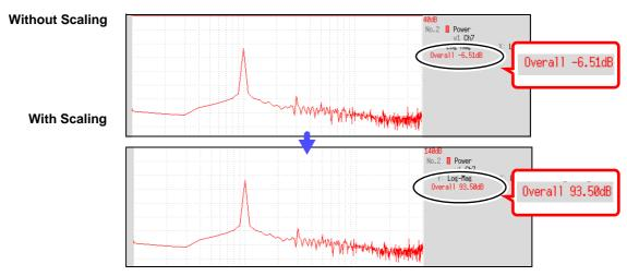
Setting example: To display measurement data on this instrument so that it corresponds to that on a sound level meter.
