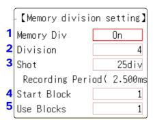
Memory Division, Waveform Calculation, and Roll Mode cannot be enabled at the same time.
