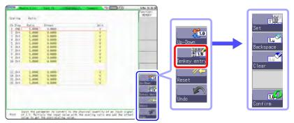
Use the virtual keyboard for numeric keypad input.
