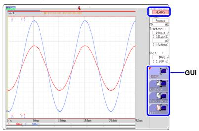
2 Check the GUI illustration and press the function key (F key) for the setting that you want to change.
