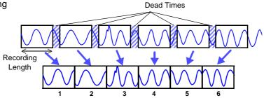
The waveform data of each recording length is recorded in one block.
