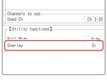
This mode cannot be used simultaneously with the Roll Mode.
