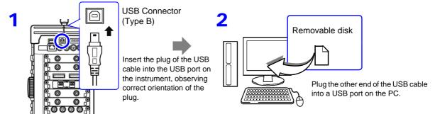
When the connection is established, the computer will recognize the instrument as a removable disk. The computer can now access data on the HDD or CF card of the instrument.
