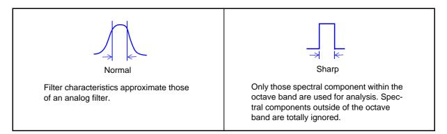
After determining the entire power spectrum, the instrument performs octave analysis on the spectral bands defined by the above filter characteristics.
