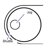
The scrolling speed is controlled by the rotation angle of the Shuttle knob.
