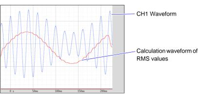
To view calculated waveforms of loaded data, move to the [Wave Calc] sheet and select [Exec].
