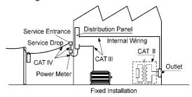
CAT III Primary electrical circuits of heavy equipment (fixed installations) connected directly to the distribution panel, and feeders from the distribution panel to outlets.
