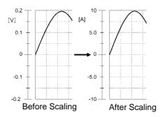
With scaling, signals from the sensor are acquired as current values.
