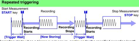
Recording starts when a trigger event occurs, continues for the specified recording length, and returns to the Trigger Wait state.
