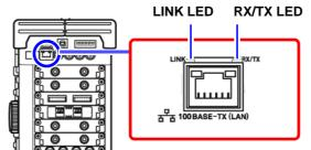
Lights while the instrument is capable of communications with a destination device.
