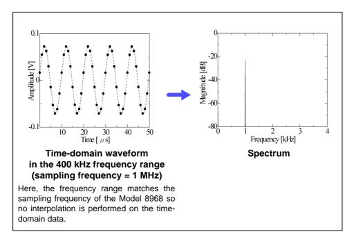
To avoid imaging phenomena when analyzing waveforms with the FFT function, verify the maximum sampling frequency of the input module before measuring.
