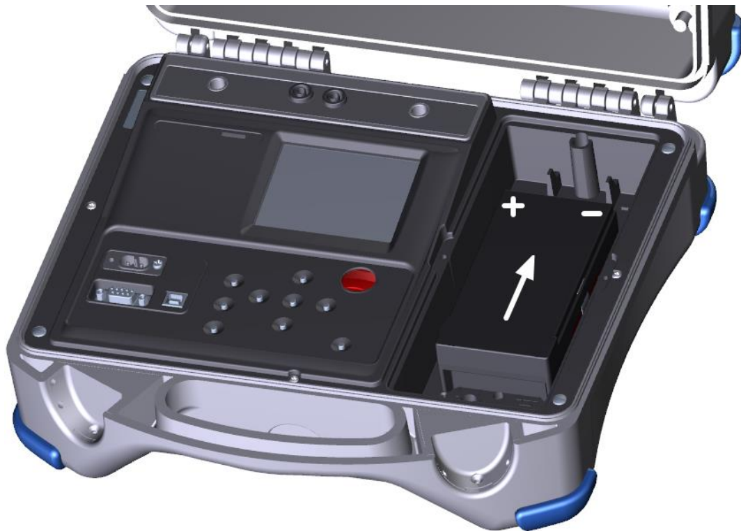
Figure 7.2: Correctly inserted battery
