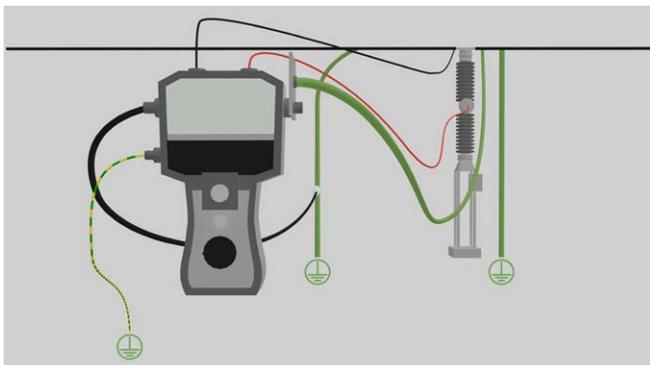
Traditional measurement from ground. Injection is done through existing grounding cable (earthing). use any of the optional cable kits, GA- 00380/82/84 with 5,10, or 15 m cables.
