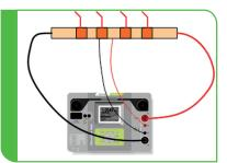
**Example 2:** Testing the **bus bar** contact resistance. By using higher currents bus bar resistance under similar condition as in normal use can be observed. This will give you more reliable result and easy decision about necessary maintenance.
