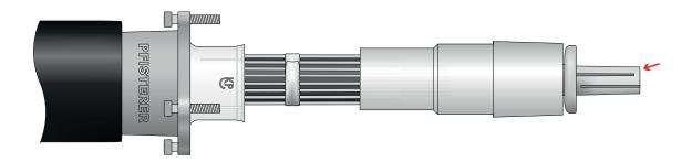
Slide the contact ring onto the tension cone.
