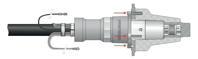
4 Pull the CONNEX termination out of the socket.
