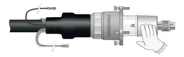
2 Clean the inside of the socket (recommended cleaning agents: benzene, acetone) and grease thinly with PFISTERER MV-special grease. Wear clean protective gloves (e.g. latex or plastic).
