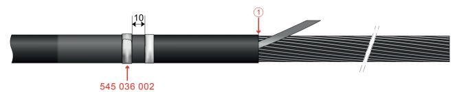
Fold back the screen wires and fix with insulating tape.
