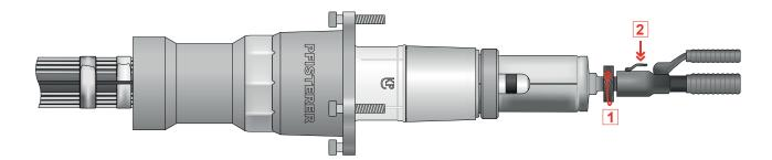
11 Pull the contact ring off the tension cone with the hydraulic compression tool.
