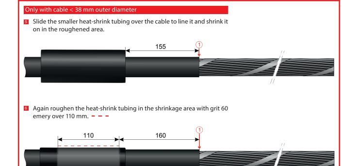
10 Apply the control mark 160 mm from the "jacket cut" (1).
