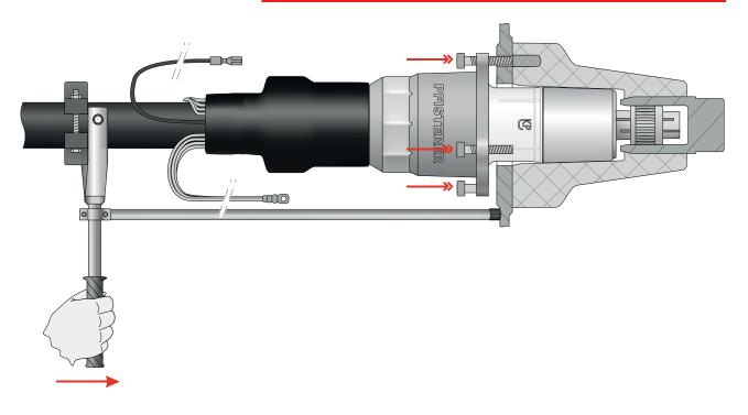
3 Clean insulating part (recommended cleaning agent: benzene, acetone) and protective cap (not voltage-proof) or blind cap (permanent) raise.
