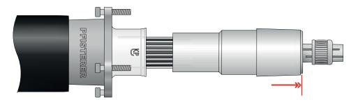
21 Slide the bell flange onto the insulating part.
