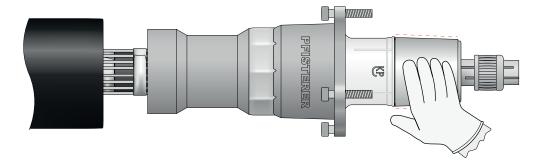
Clean the surface of the socket (recommended cleaning agents: benzene, acetone) and grease thinly and evenly with PFISTERER MV-special grease. Wear clean protective gloves (e.g. latex or plastic).
