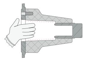
Introduce the CONNEX separable connector into socket and tighten the screws.
