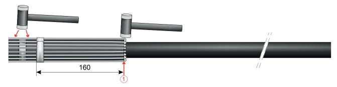
Mark end of the cable 300 mm from the "jacket cut" (1) for a provisional cut and saw off straight with a hacksaw.
