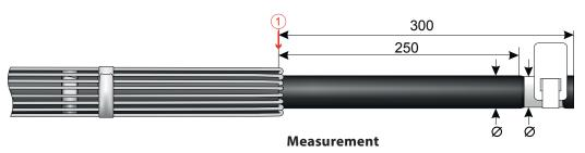
Ø semi-conductive layer - Ø insulation = Ø difference
