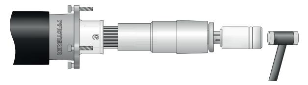
III Slide the retaining ring of the compression head back and fix the half-shells behind the thrust piece.
