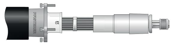
Fix contact ring onto the tension cone with the impact head. The contact ring must no longer be able to rotate.
