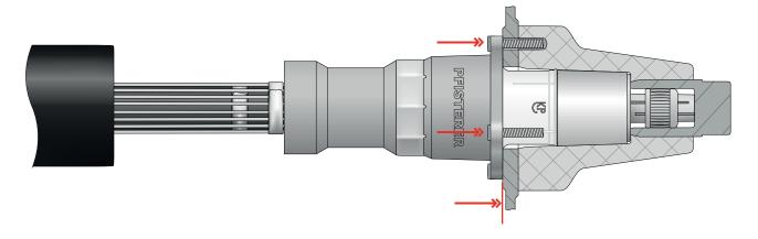
Using the ruler, check the position of the control dimension 207 mm. If not acheived press the cable again. **Do not remove the check mark!**
