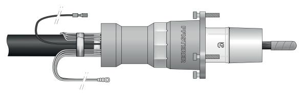
Remove the insulating part and bell flange.
