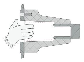
Introduce the CONNEX separable connector into socket and screw in the screws.
