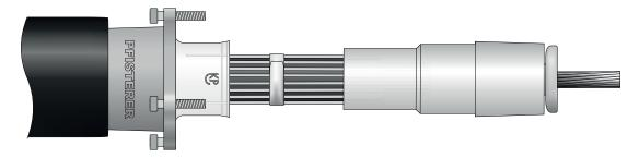
II Slide the tension cone onto the conductor up to the thrust piece.
