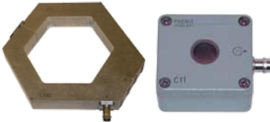
When a current transformer is used instead of a quadrupole, the current transformer can be placed around a coupling capacitor terminal or around a part of the test object itself. A current transformer has the advantage of providing galvanic isolation between the PD detector and the high voltage circuit. Current transformers are offered as separate modules or integrated with a coupling capacitor into a single unit.
