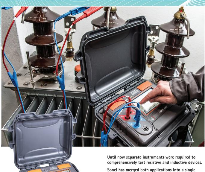
Sonel has merged both applications into a single economical and compact instrument with the new Li-lon powered 10 Amp MMR-650.
