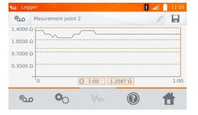
Use button to display the graph of resistance over time both during the logging process and after its completion.
