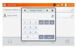
Enter the lower limit. Use button to go to the upper limit setting. You can set only one of the limits.
