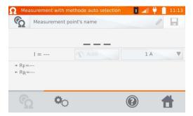
The measurement is performed as in the case of testing the inductive objects If based on the difference between the instantaneous and average resistance during the result stabilization, the meter determines that the object is resistive, it will complete the measurement faster.
