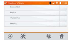
The meter has 4 default types saved in its memory. Use to button to add a new type of the tested object.
