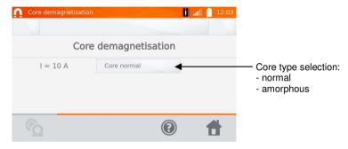
Connect the meter to the transformer windings. Press START/STOP. Wait for the following screen.
