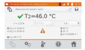
$R_{\text{T1}}$  – resistance of the cold winding
