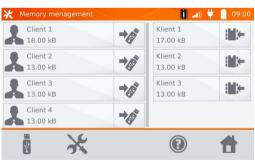
Click, to save data in the USB stick or to copy data from the USB stick to the memory of the meter.
