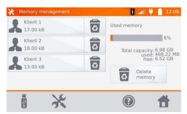
This option allows you to read the % of the used memory and to clear it: after pressing **Delete memory** all clients are deleted with their objects and measurement results. Use
