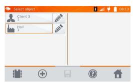
After adding and saving the object (also subobjects if necessary), click button to add the measurement point.
