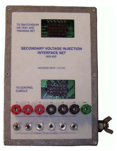
The maximum voltage that can be applied to the SVIIS is 110 VAC.
