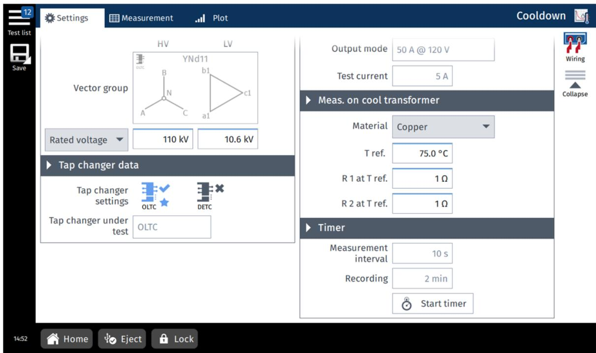
Figure 8-23: Cooldown test – **Settings** view
