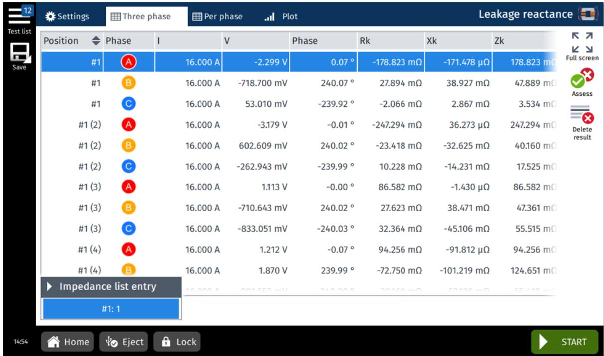
Figure 8-10: Short-circuit impedance test – **Measurement** view
