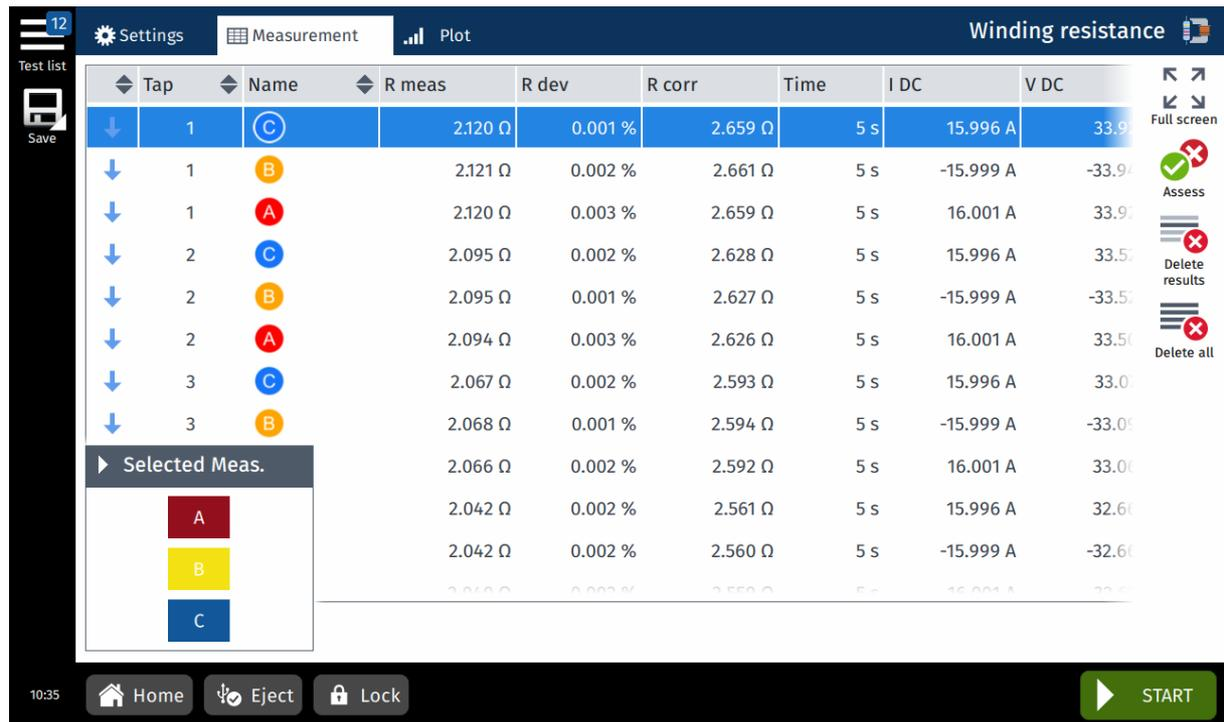
Figure 8-6: Winding resistance test – Measurement view
