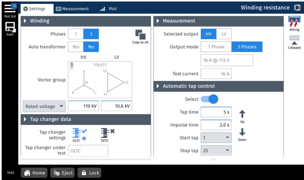
Figure 8-5: Winding resistance test – **Settings** view
