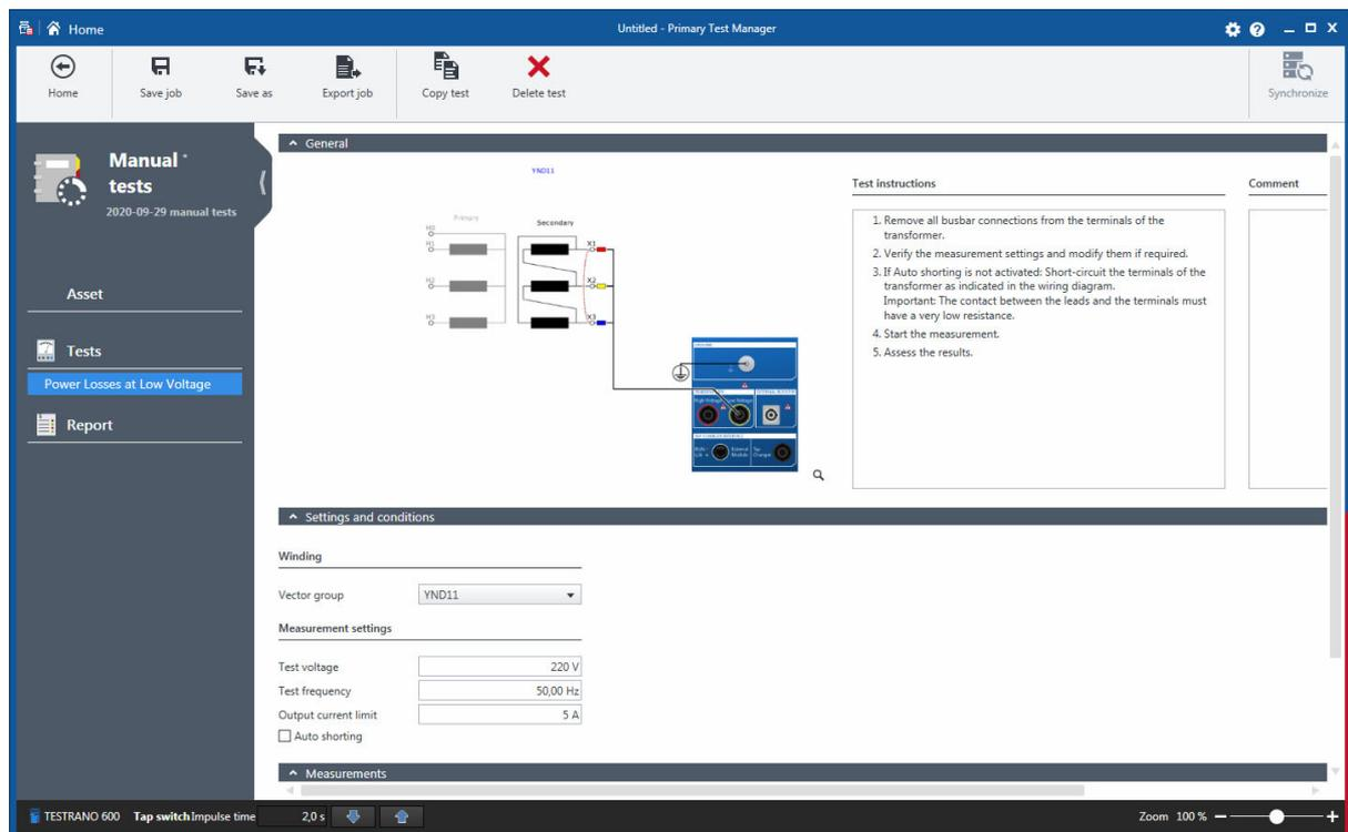
Figure 12-9: Power losses at low voltage test
