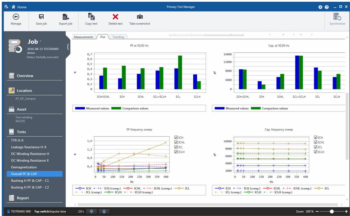
Figure 9-40: Test comparison: Measurement results of both tests
