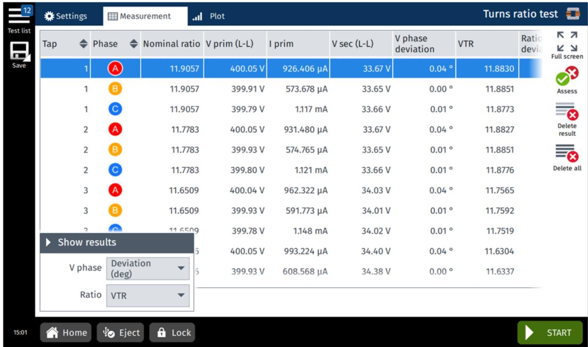
Figure 8-4: Turns ratio test – **Measurement** view with results
