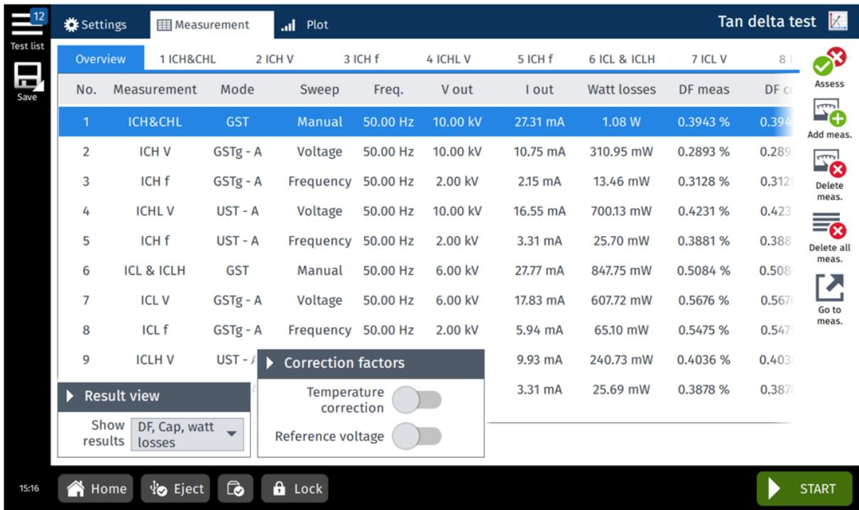
Figure 8-12: Tan delta test – Measurement view
