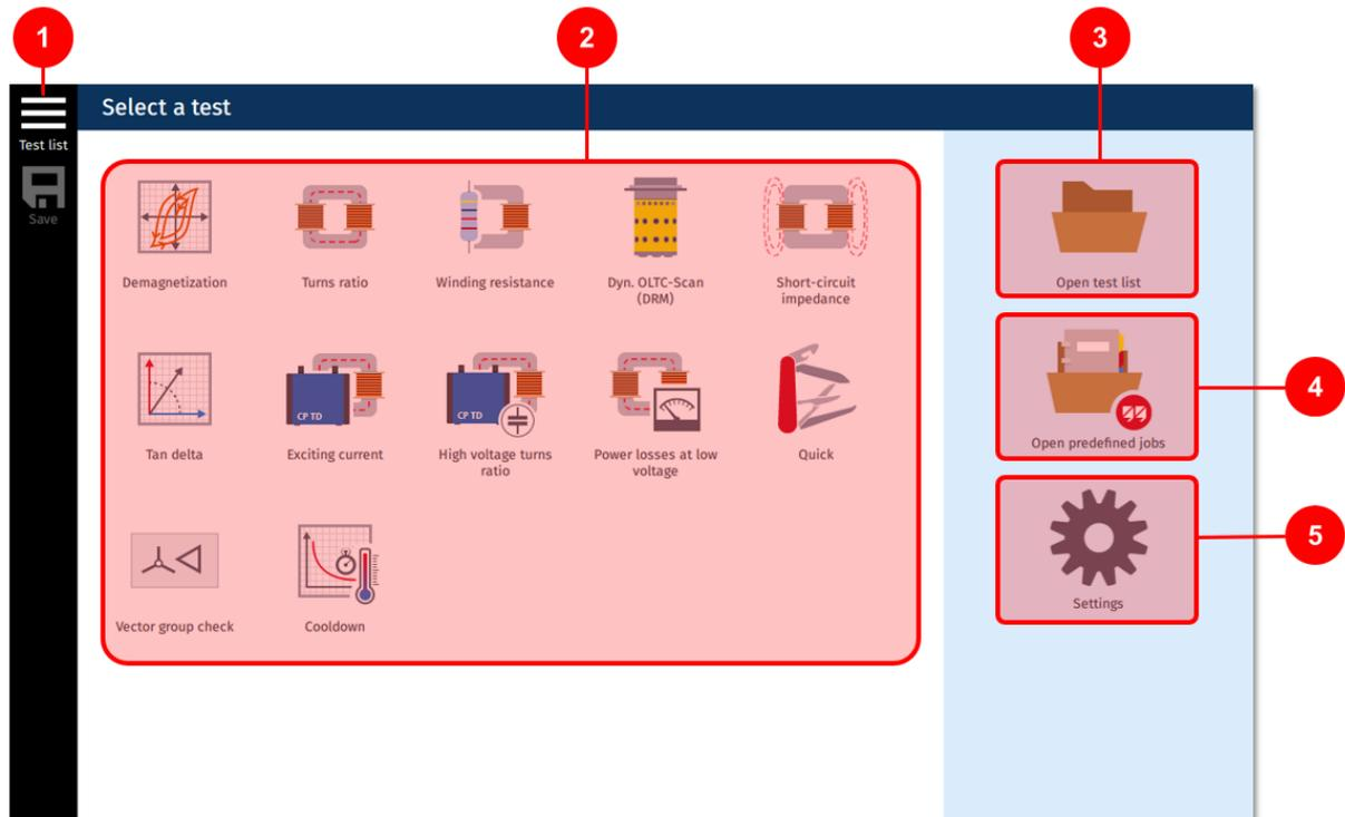
Figure 6-1: *TouchControl* – **Select a test** view
