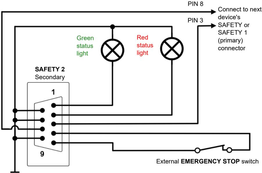
Figure 15-9: SAFETY 2 (secondary) connector schematics
