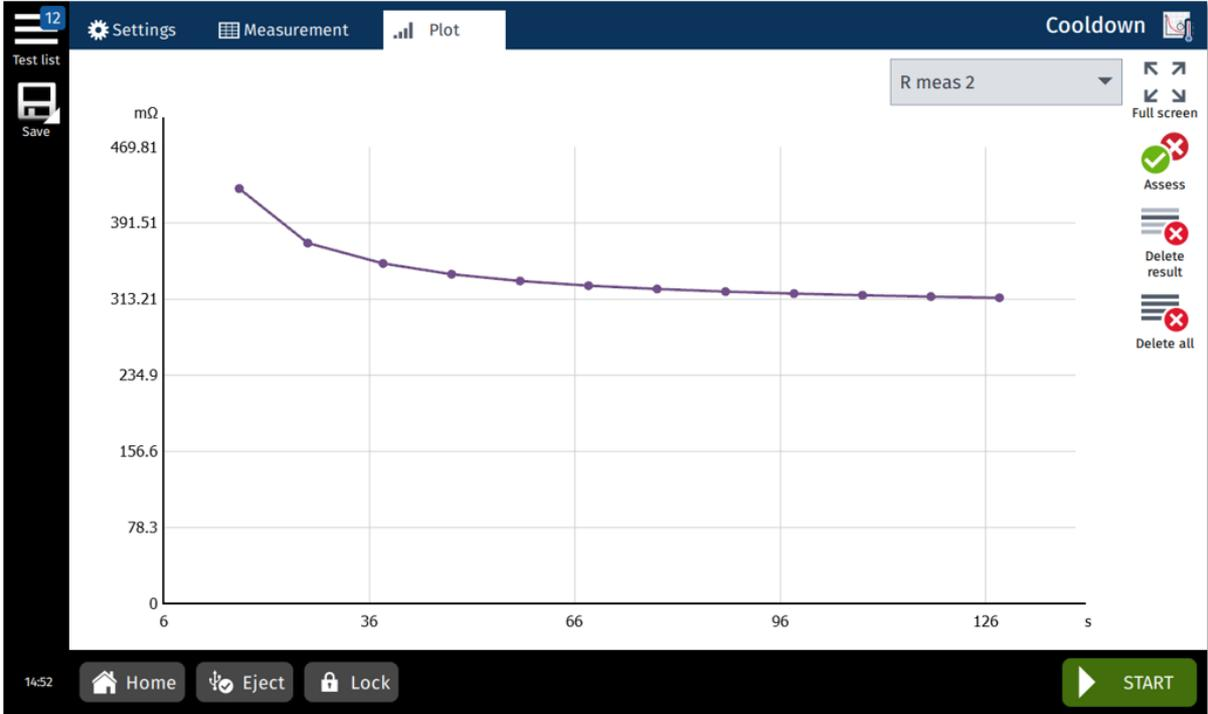
Figure 8-24: Cooldown test – Measurement view
