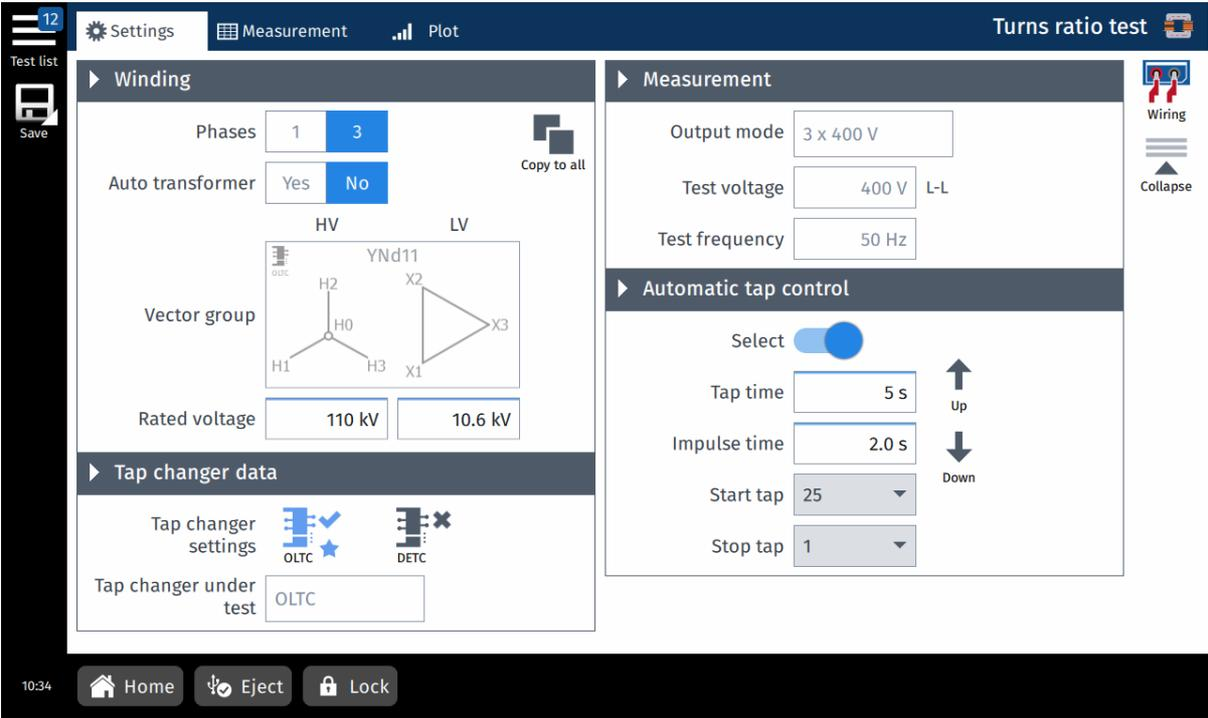
Figure 8-3: Turns ratio test – Settings view
