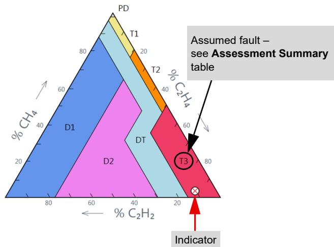
Key gas ranges and conditions according to IEC 60599, visualized in 3D
