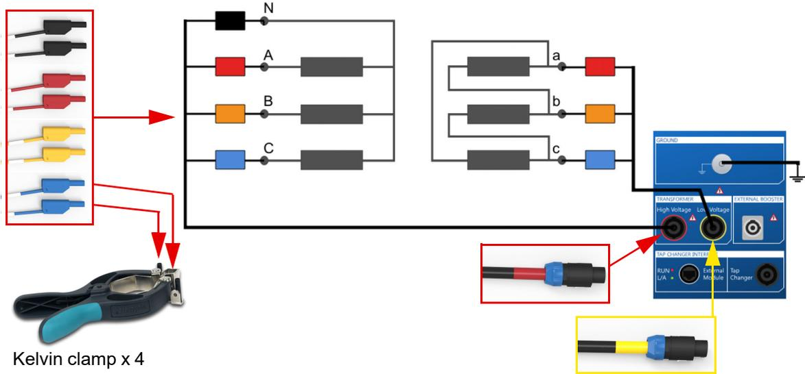
Figure 7-2: Wiring diagram for a TTR (Turns Ratio Test) on a transformer with the vector group YNd5
