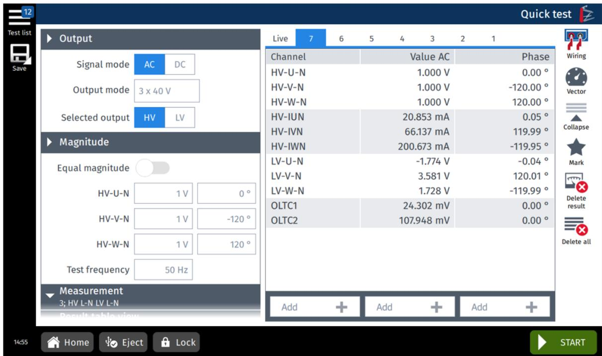
Figure 8-20: Quick test – **Measurement** view (table form)
