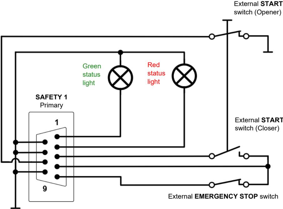
Figure 15-8: SAFETY 1 (primary) connector schematics
