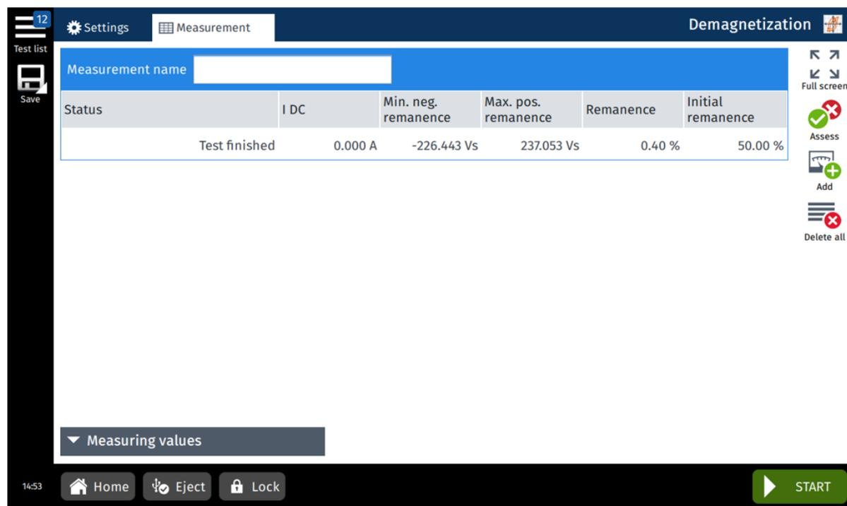
Figure 8-2: Demagnetization test – **Measurement** view
