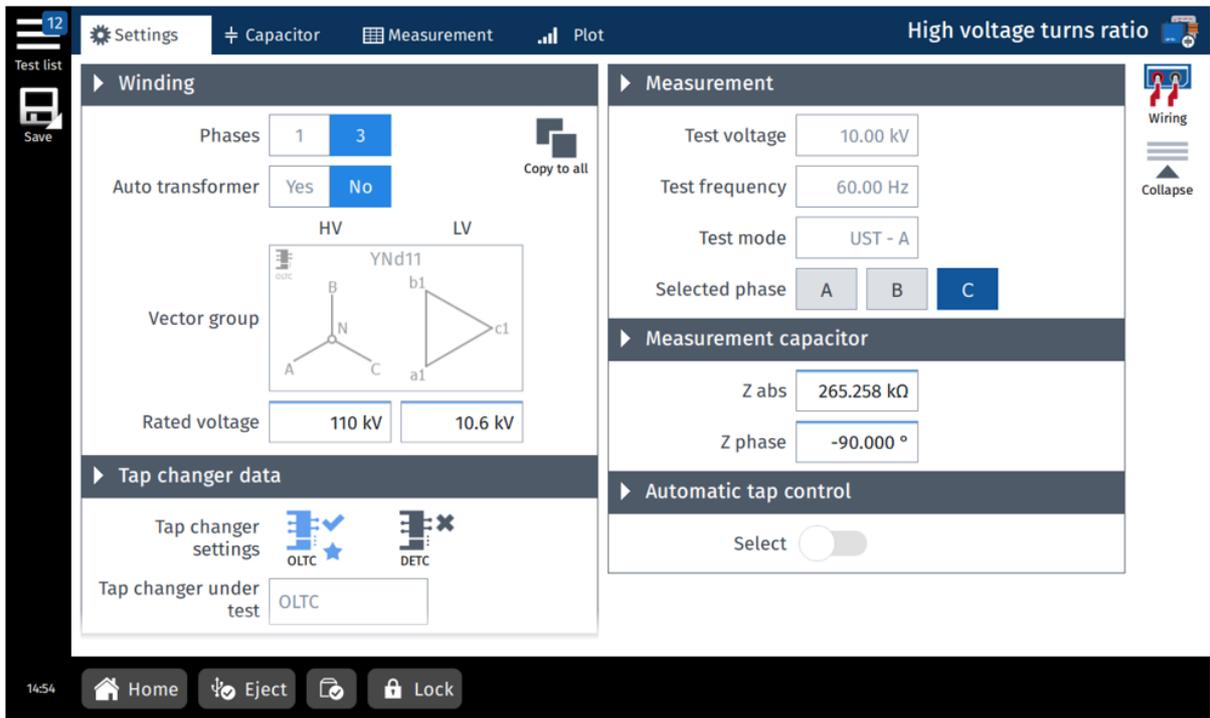
Figure 8-15: High voltage turns ratio test – **Settings** view
