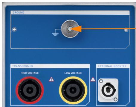
Connect the *TESTRANO 600* grounding terminal to the grounding system on site.
