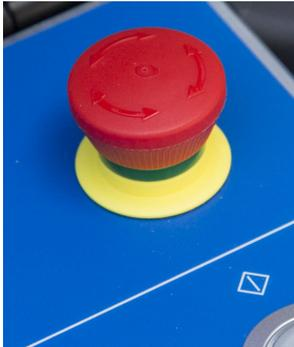
Pressing the **Emergency Stop** button *immediately* shuts off all *TESTRANO 600* outputs and stops the running measurement. When the **Emergency Stop** button is pressed, you cannot start any measurements.
