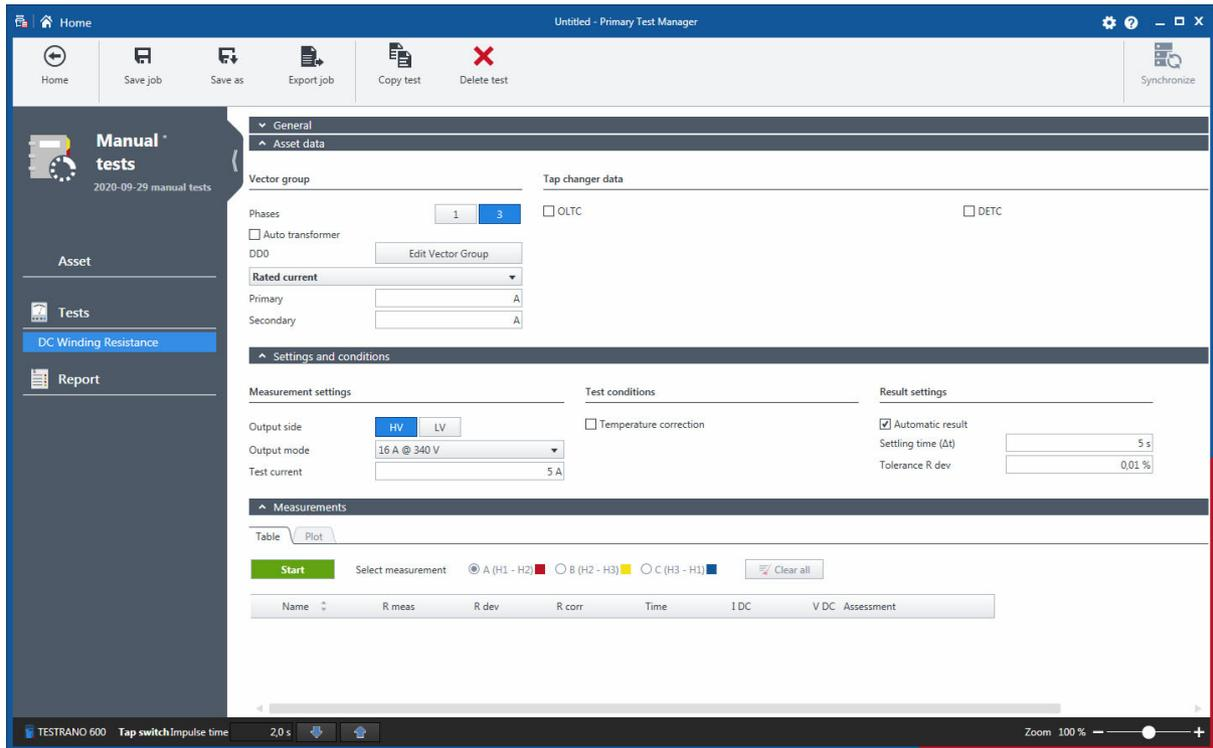
Figure 12-13: Manual DC Winding Resistance test
