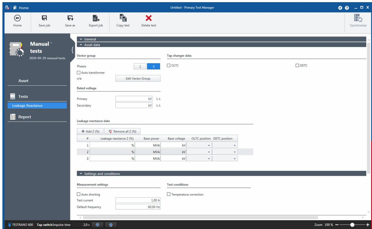
Figure 12-15: Manual Leakage Reactance test
