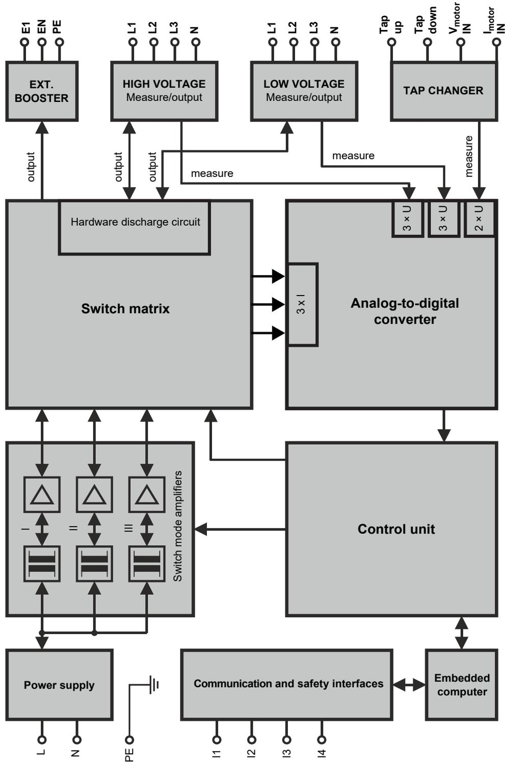
Figure 4-1: Functional scheme for TESTRANO 600
