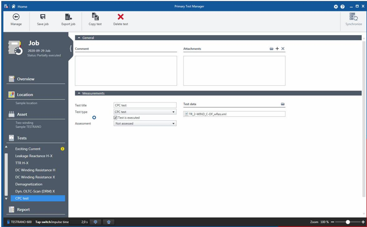
Figure 9-30: Test view after a test has been imported
