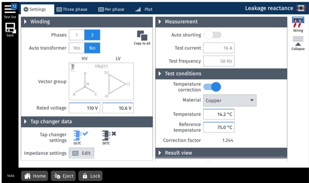
Figure 8-9: Short-circuit impedance test – **Settings** view
