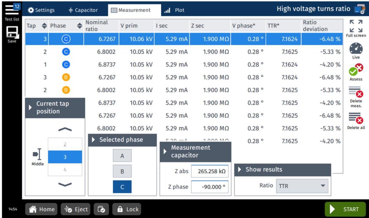
Figure 8-16: High voltage turns ratio test – **Measurement** view with results
