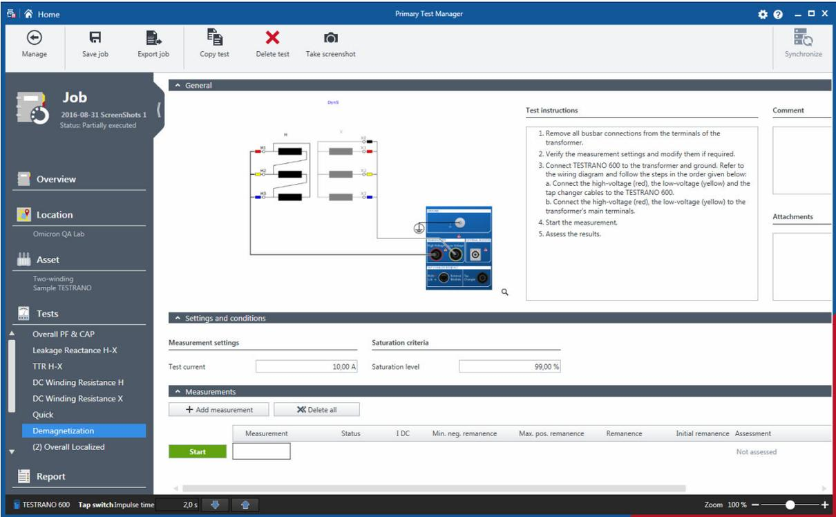
Figure 12-7: Demagnetization test view
