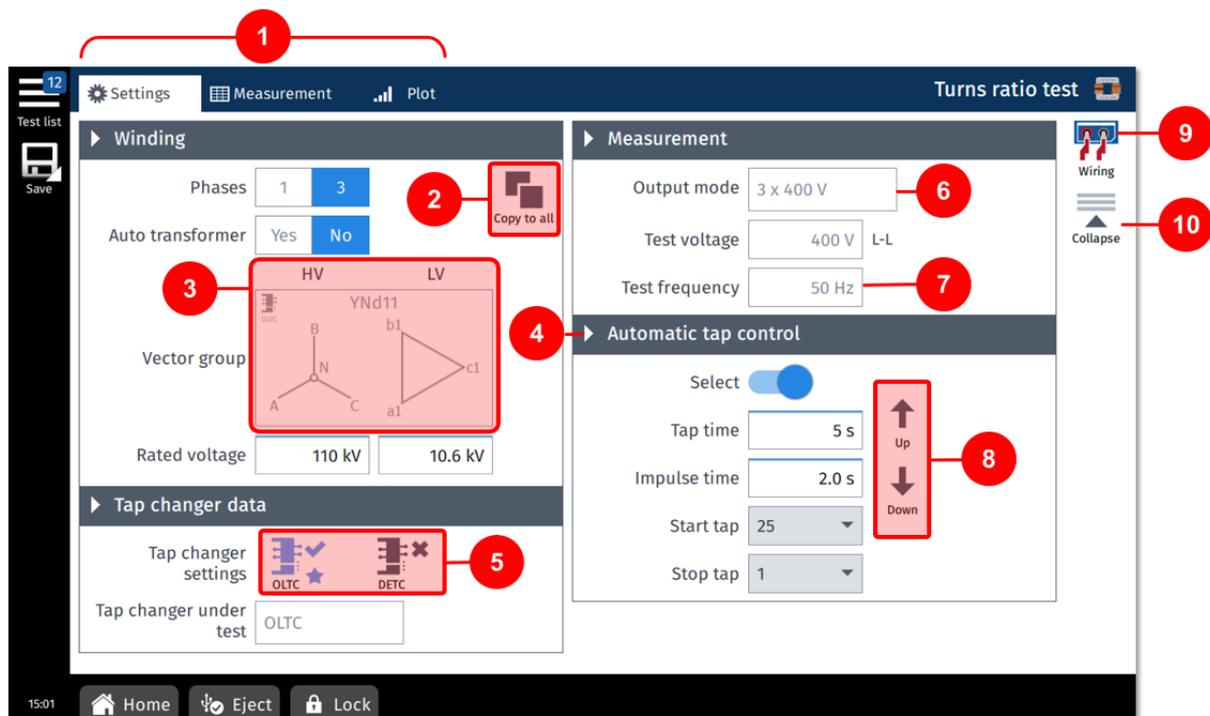
Figure 7-1: Example of a **Settings** view - **Turns ratio** test
