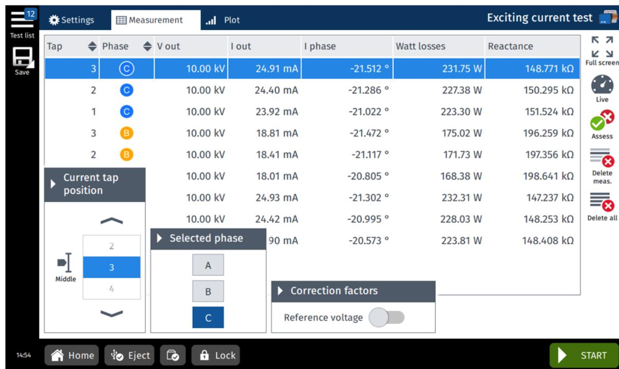
Figure 8-14: Exciting current test – Measurement view
