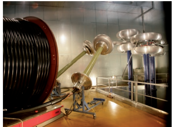
Factory test of a cable drum
