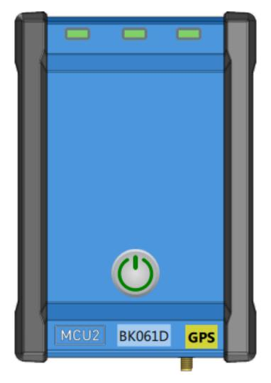
Figure 14.3: MCU 2 with GPS fix and no synchronization
