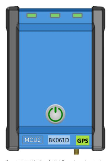
Figure 14.4: MCU 2 with GPS fix and synchronization
