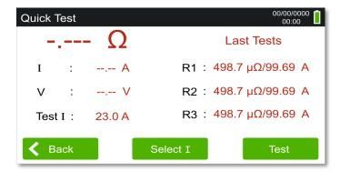
Press the 'Select I' tab to select the test current.
