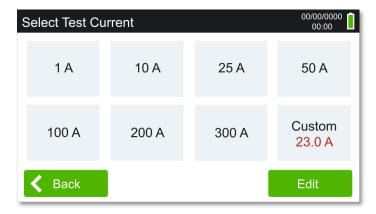
Users can choose test current options available on the device or manually enter a value on the custom tab.
