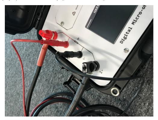
Connect the test cables to the sample to be tested as shown in the figure below and press 'Quick Test' tab.
