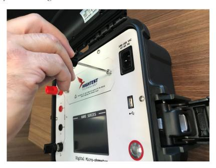
2. Remove the battery from the device carefully.
