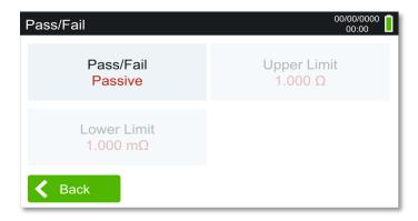
Users can set an upper and lower limit to compare the results they obtained during the tests. To achieve this, make the Pass/Fail tab 'Active'.
