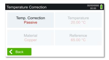
Users can set a reference temperature to get temperature corrected test results. To, achieve this, make sure to make the Temp. Correction tab 'Active' and select the appropriate material and set the reference temperature.
