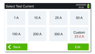
The device comes with certain range of test current from which a user can choose. 200A and 300A are only available to HARE-200 and HARE-300 devices. For other values, users can manually add according to their require. However the value must be under or equeal to the maximum test current value as per the technical specification of the device. The customized value can be entered by the numerical keyboard of the device by pressing 'Custom' tab.
